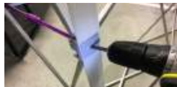
4. Secure the female arm by screwing the plate to the frame hub.
